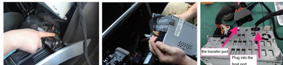
Complete the transfer of air conditioning panel
